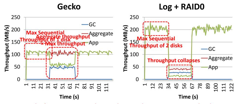
Gecko's aggregate throughput always remains high 3X higher aggregate & 4X higher application throughput
